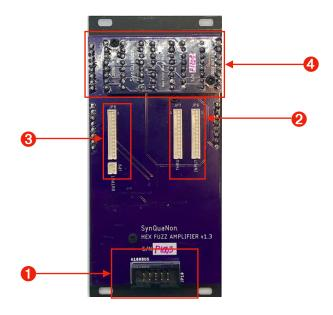
1 A100 Bus Keyed power connection with reverse polarity protection.
