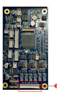
A100 Bus Keyed power connection with reverse polarity protection.
